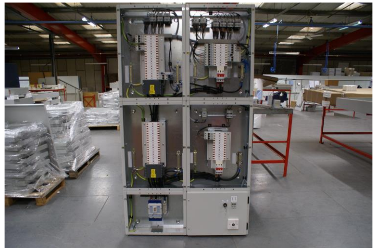
Switch panel under construction in Proteus, Telford.
